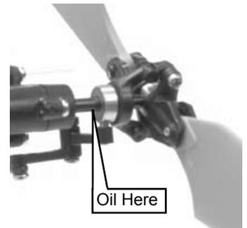
Place a tiny bit of oil (any good lubricant for metal on metal) on the tail output shaft. This will keep the tail pitch slider sliding smoothly on the output shaft.
