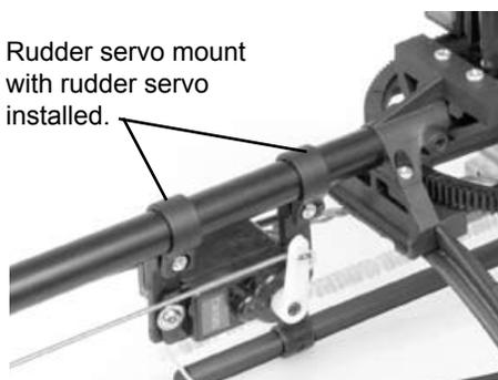
The servo arm should be positioned for maximum travel range. setting the servo arm at a 90 degree angle to the tail boom will give equal (maximum total) travel distance on both ends of the servo travel range.
