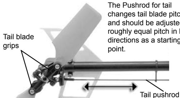
The only way to get perfect tail control is to test your settings and adjust until the helicopter responds equally for both directions of rudder control. Keep in mind that the tail is compensating for main rotor torque. Note: main rotor torque turns the helicopter counter-clockwise.
