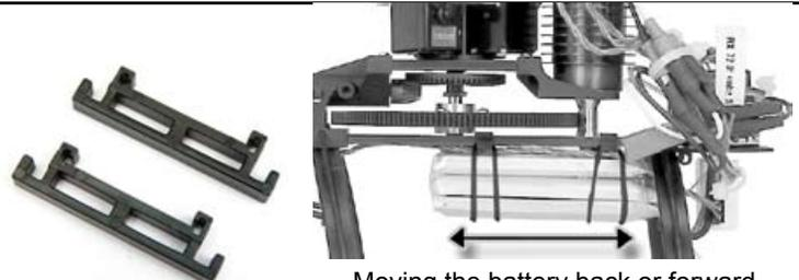
Moving the battery back or forward will help adjust center of gravity
